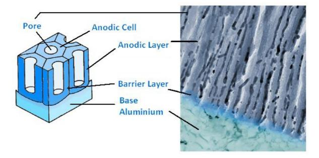
Did you know? Aluminium Oxide  $(Al_2O_3)$  is also known as Corundum. Gem varieties of Corundum include Ruby, Sapphire, & Emery. Among the natural gems only Diamond is harder than Corundum. This explains why the Anodised Aluminium surface is so hard!
