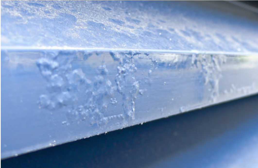
Appendix B: Examples of powder coating that has failed in the field after less than 6 months. Coated by another coater who does not have proper, nor Qualicoat Standard Pre-treatment for Aluminium.
