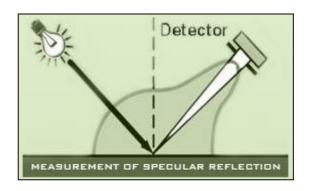
Gloss of a surface is not a unique physical property. It varies with the angle of measurement; it is not independent of the apparatus being used. The 60° geometry is the "universal measurement angle". Due to its medium gloss coverage, it is widely used and applicable for surfaces with Gloss values of between 10 & 70 Gloss Units (GU).
