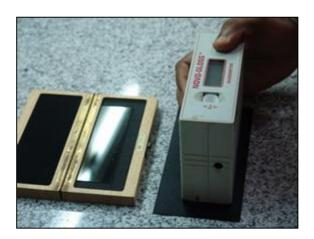
As an example, this means that a measurement of "40 GU" means that the sample reflects 40% as much light as the black glass standard. That is not to say that it reflects 40% of incident light. It also means that sample measurements of >100 GU are possible, implying that the sample is more reflective than the black glass standard.
