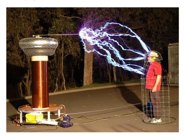
In day-to-day application, this phenomenon is not visible. However, in a recent scale up version of Faraday's experiment, it can be seen in the above photo, that the man is protected from the electric arcs by the "Faraday cage".
